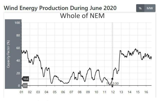
**The drought of the 5**<sup>th</sup> **to 6**<sup>th</sup>. The wind was below 10% of capacity for a period 33 hours. In South Australia, New South Wales and Victoria the wind stopped completely for many hours during this period and for some of the time the turbines drew power from the grid instead of contributing to it!
